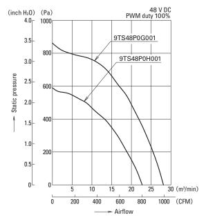
Fig. 8: Airflow vs. static pressure characteristic of the "San Ace C225" 9TS type
