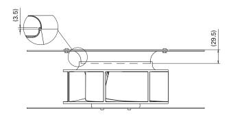
Fig. 6: Example of the "San Ace C225" 9TS type and inlet nozzle mounting dimensions (unit: mm)
