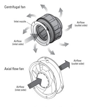
Fig. 12: Airflow of a centrifugal fan and an axial flow fan
