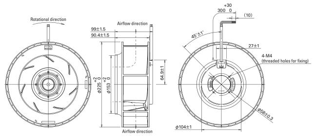
Fig. 3: "San Ace C225" 9TS type dimensions (unit: mm)
