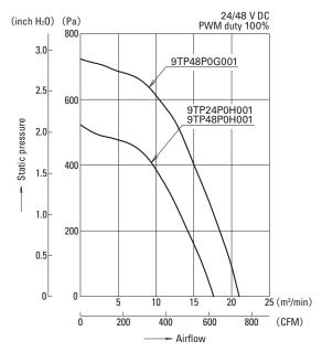
Fig. 9: Airflow vs. static pressure characteristic of the "San Ace C221" 9TP type
