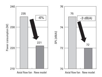
Fig. 11: Comparison of power consumption and SPL
