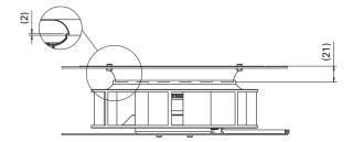
Fig. 7: Example of the "San Ace C221" 9TP type and inlet nozzle mounting dimensions (unit: mm)
