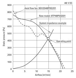
Fig. 10: Comparative example of the airflow vs. static pressure characteristic
