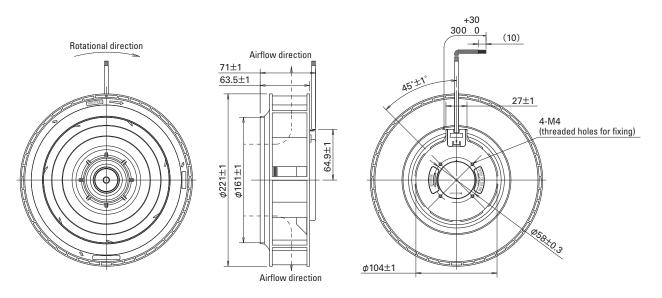
Fig. 4: "San Ace C221" 9TP type dimensions (unit: mm)
