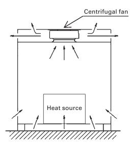
Fig. 13: An example of centrifugal fan usage
